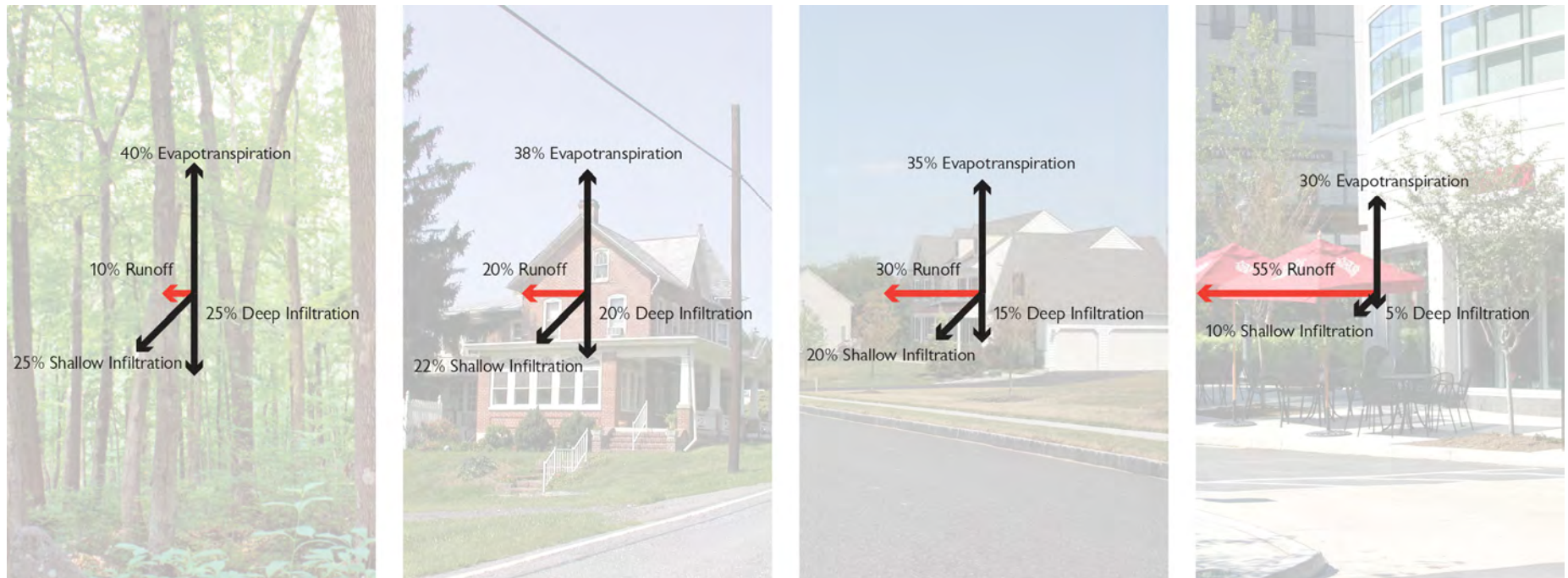
FIGURE 117: Impacts to the Hydrologic Cycle from Development
